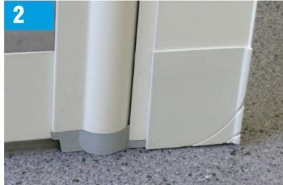
If fitting your enclosure on a wet floor, a corner block at the base of each compensator can be shaped at 10mm or 38mm radius to accept floor covering. Cut along the pre-formed indents.
