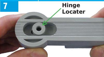
Our **NEW** 2 part rise & fall hinge has been designed to make our doors more stable. The hinge locator screws to the tray or floor and will fit into the centre of the recess underneath the hinge, as demonstrated above.
