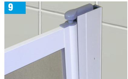
Offer the door(s) back into their respective compensators, re-align with the mark(s) you had previously made for the door position. **ENSURE** the compensator is fixed securely to the wall. Use the supplied hinge locator, FIG 7 & 8, if necessary for added rigidity.
