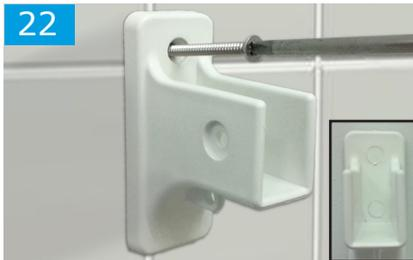
Drill the wall with a No10 masonry drill, insert wall plugs and fix with 2" countersunk self tapping screws. Use the supplied blanking caps to cover the screw heads, see inset.
